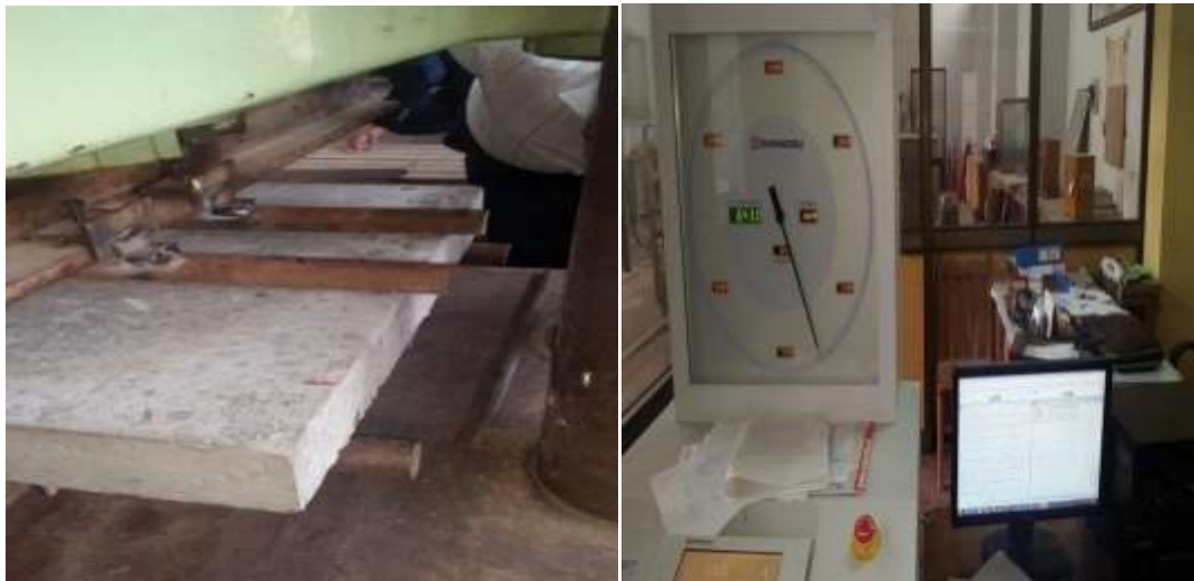
Figure (6) Test of flexural strength experimental setup
